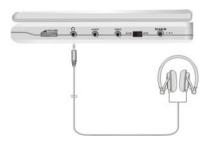
When headphone is connected, the speakers will automatically turn off.
